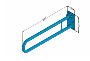
Handrail for disabled people, arched, tilting, wall-mounted, length 800 mm, general-purpose, made of 32 mm diameter carbon steel tube, black powder coated. We use this type of handrail in the washbasin, shower, and toilet area.
