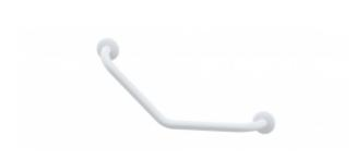
Angled handrail made of white powder-enameled carbon steel (anti-corrosion primer was used for enameling). The 350x350 handrail is intended for wall mounting in the bathtub area. The diameter of the tube used in the production is 32 mm, while the wall thickness is 1.5 mm. The maximum load capacity of the railing is 180 kg.
