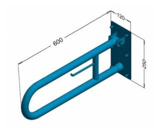
Tilting arch handrail with a place for toilet paper for disabled people, length 600 mm, general-purpose, made of polished stainless steel tube or matte 32 mm diameter. We use this type of handrail in the wc area.
