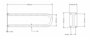
**Arched and tilted handrail for the diabled**, makes everyday actions easier and rises safety for **eldery and disabled** people. While using sanitary products like shower, washbasin or toilet. handrail for disabled is made of ø25 mm tube (thicness 1,5 mm), made of stainless steel AISI 304. It hac PZH and CE certificate and entry in the register of medical devices. Max. weight is 180 kg. For general use
