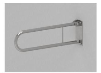
Arched and tilted handrail for the diabled, makes everyday actions easier and rises safety for **eldery and disabled** people. While using sanitary products like shower, washbasin or toilet. handrail for disabled is made of ø25 mm tube (thicness 1,5 mm), made of stainless steel AISI 304. It hac PZH and CE certificate and entry in the register of medical devices. Max. weight is 180 kg. For general use
