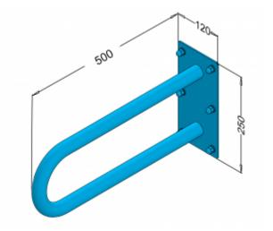
Arch fixed wall for disabled people, length 500 mm. generalpurpose, made of polished stainless steel tube or matt 32 mm diameter. We use this type of handrail in the washbasin, shower, and toilet area.
