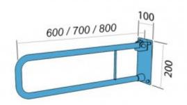
Handrail for disabled people, arched, tilting, wall length 800 mm, general-purpose, made of 25 mm diameter carbon steel tube, white powder coated. We use this type of handrail in the washbasin, shower, and toilet area.
