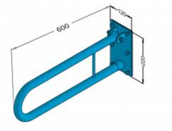
Handrail for disabled people, arched, tilting, wall-mounted, length 600 mm, general-purpose, made of 32 mm diameter carbon steel tube, white powder coated. We use this type of handrail in the washbasin, shower, and toilet area.
