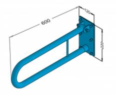
Handrail for disabled people, arched, tilting, wall-mounted, length 600 mm, general-purpose, made of 32 mm diameter carbon steel tube, black powder coated. We use this type of handrail in the washbasin, shower, and toilet areas.
