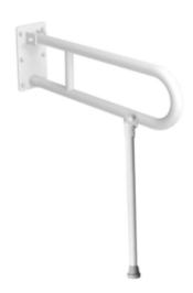
Handrail for disabled people, arched, tilting, wall-mounted, length 600 mm, general-purpose, made of 32 mm diameter carbon steel tube, white powder coated. We use this type of handrail in the washbasin, shower, and toilet area.
