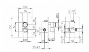
Concealed shower tap with progressive mixer and ceramic cardrige. The outer part of the faucet is made of brass covered with a shiny chrome layer. In the central part of the body there is a button that starts the flow of water and a lever that regulates the water temperature. The offered valve has a built-in progressive mixer with two G1 / 2 connections for cold and hot water.
