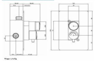
Shower timer with thermostatic mixer. Temperature regulation by means of a knob located below the start button. Possibility of safe water temperature regulation thanks to anti-scalding protection preventing exceeding the permissible temperature of 38°C. A single water flow can last 15-25 seconds (water pressure 3 bar), with water consumption of approx. 6 l / m. The water connection pressure can be 0.5 - 6 bar, however, the recommended connection pressure should be 2-4 bar.
