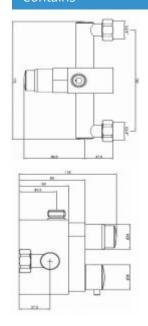
Wall-mounted shower timer with ceramic mixer for cold and hot water. Temperature control with the knob below the start button. The 5008N faucet is made of brass covered with a layer of chrome. One-time flow of water takes about 15 - 25 seconds.
