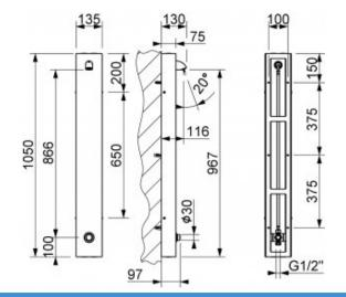
Self-closing shower panel with G1/2 connection for cold or mixed water. The faucet head is made of brass, while the rest of the panel is made of stainless steel.
