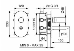
The 8351 tap is made of corrosion-resistant brass covered with a chrome layer. The 8351 faucet has one G3/4 connection. A single water outflow, with the standard setting of the faucet, is about 15 seconds  $\pm$  3 seconds. The connection pressure can range from 0.5 bar - 6 bar, however, the recommended pressure is 2-4 bar. The 8351 tap uses anti-scaling parts with a built-in anti-calc system.
