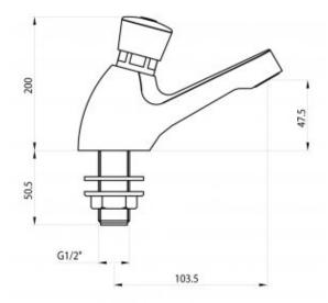
The 9001 basin tap is a classic product for mixed water. The body is made of solid brass covered with chrome. The whole has one G1 / 2 connection and elements regulating the water flow. The mentioned elements are:
