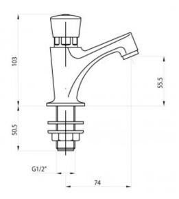
The 9002 basin tap is a classic product for mixed water. The body is made of solid brass covered with chrome. The whole has one G1 / 2 connection and elements regulating the water flow. The mentioned elements are:
