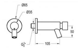
The time battery, adapted for wall mounting with a button, is a product designed for public spaces, such as shopping centers, spas, hospitals, swimming pools, and others. The body of the faucet is made of brass with a black finish.
