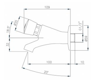
Wall-mounted washbasin timer with one G1/2 connection for cold or pre-mixed water. The body of the faucet is made of solid brass covered with a layer of chrome. The built-in spout is equipped with a standard strainer to regulate the water stream.
