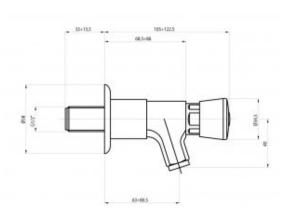
Wall-mounted washbasin timer with one G1 / 2 connection for cold or premixed water. The body of the faucet is made of solid brass covered with a layer of chrome. The built-in spout is equipped with a standard strainer to regulate the water stream.
