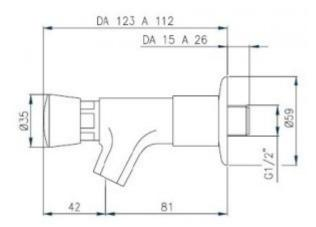
Self-closing wall-mounted timer tap with one 1/2" connection for cold or mixed water. Used in rooms equipped with premixed water supply. The faucet is equipped with a lever for easy operation, e.g. for the disabled or for children. Moreover, the mixer is made of brass covered with chrome and has a 15-year warranty.
