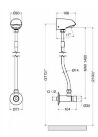
Self-closing shower set with a fixed spout mounted to the wall. The supply pipe has a diameter of 14 mm and, what is important, the mounting is fitted to wall mounting. The shower set has one 1/2 &HASH39; connection for cold or mixed water, with a standard water flow time of about 30-50 seconds ± 1 second. The flow system is enriched with a safety device that automatically shuts off the water flow after 15 seconds (at a pressure of 3 bar).
