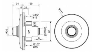
Shower tap for concealed installation. The tap has one G1 / 2 connection for cold or mixed water. The body of the faucet is made of stainless steel AISI 316L. A single outflow of water in the 9005 shower tap takes about 15 - 25 seconds.
