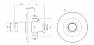
Shower tap for concealed installation. The tap has one G1 / 2 connection for cold or mixed water. The body of the faucet is made of brass covered with a layer of chrome. A single outflow of water in the 9005PLUS shower tap takes about 15 - 25 seconds. The amount of water consumed at the outlet is approx. 6 l / m, at a water connection pressure of 3 bar. The connection pressure can be from 0.5 to 6 bar, however the recommended connection pressure should be from 2 to 4 bar.
