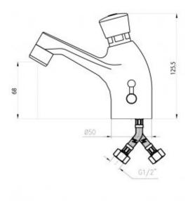
The washbasin timer with an integrated mixer and aerator a reliable product most often used in public spaces. The 9007 faucet is made of corrosion-resistant chrome-plated brass. In the side part of the body there is a mixer, regulated by a lever.
