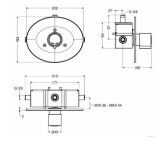
The self-closing flush-mounted mixer with 3/8 &HASH39; connections for cold and hot water is a product that was made of chrome-plated brass and that is adapted for wall mounting for shower cabins. The self-closing cartridge is activated by a button located in the central part of the mixer. Mixer 9010MIX is available in two mounting variants:
