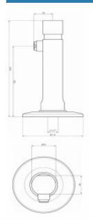
Washbasin, wall-mounted, cold or mixed water timer. Used in rooms with pre-mixed water supply. The modern design makes the tap ideal for high-standard places. The 9073 faucet is made of chrome-plated brass and has one G1 / 2 connection.
