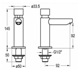
The self-closing basin tap with a moving aerator. The body is made of AISI 316 stainless steel. The tap has one G1 / 2 connection. A single outflow of water takes about 15 seconds (at a water pressure of 3 bar). The amount of water used is 5 l / m. The minimum connection pressure is 1 bar, the maximum is 5 bar. It is worth adding that the recommended connection pressure should be 2-4 bar.
