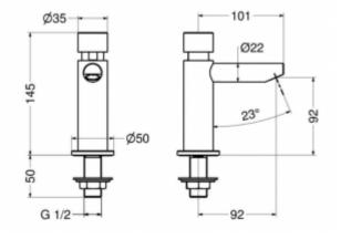
A time button faucet made of chrome-plated brass is a device adapted to public spaces - including hotels, shopping malls, public toilets and others. The 9800 tap is equipped with one 1/2 &HASH39; connection for cold or mixed water. The water flow can be started by pressing the button on the upper part of the body. One-time water flow time is approximately 15 seconds  $\pm$  5 seconds (at a water pressure of 3 bar). What&HASH39;s more, the 9800 battery was entirely made in the European Union.
