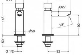
The self-closing basin tap with a moving aerator. The body is made of AISI 316 stainless steel. The tap has one G1 / 2 connection. A single outflow of water takes about 15 seconds (at a water pressure of 3 bar). The amount of water used is 5 l / m. The minimum connection pressure is 1 bar, the maximum is 5 bar. It is worth adding that the recommended connection pressure should be 2-4 bar.
