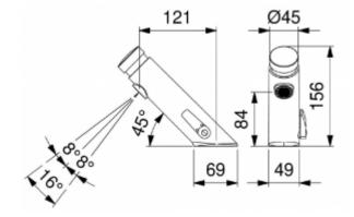
The washbasin tap with an integrated mixer for cold and hot water. The 8147 faucet is made of corrosion-resistant chrome-plated brass. In the side part of the body, there is a mixer, regulated by a
