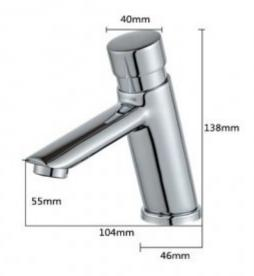
Washbasin time tap with one G1/2 connection, for cold or mixed water. The faucet body is made of brass covered with a chrome layer. There is an aerator in the spout. A single flow of water during start-up lasts 7 seconds +/- 3 seconds.
