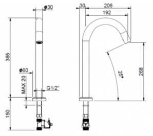
The electronic washbasin faucet with a G1/2" connection is a modern solution based on touchless operation using a built-in photocell. Equipped with an aerator, it limits water flow to 2 l/min, allowing for economical use. To maintain hygiene, the 2517B faucet is equipped with an Anti-Legionella system, which automatically initiates a cleaning cycle every 24 hours after the last use. The unit is powered by four AA batteries.
