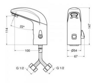
Touchless washbasin faucet with a built-in mixer for cold and hot water. The side lever allows you to adjust the temperature or allows you to set a constant water temperature. The body of the offered fittings includes an infrared sensor that activates when hands are detected. Such a system guarantees a high level of hygiene and safety of use. The 2512 series offers two power options:
