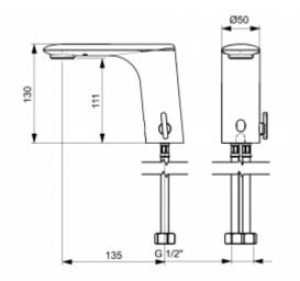
Touchless washbasin faucet with a built-in mixer for cold and hot water. The side lever allows you to adjust the temperature or allows you to set a constant water temperature. The 2514 Series offers two power options:
