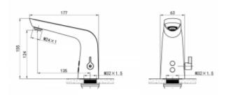
Contactless tap. Possibility to conect hot, cold and pre-mixed water. Possibility of smooth water temperature Designed for public facilities and homes.
