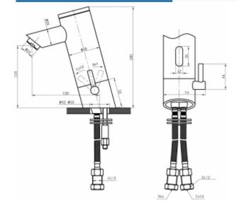
Contactless stainlees steel battery. Possibility to conect hot, cold and pre-mixed water. Possibility of smooth water temperature Designed for public facilities and homes.
