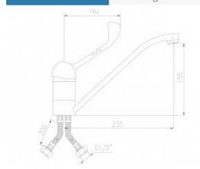
Medical mixer for hot and cold water. Used in outpatient clinics, doctor&HASH39;s offices and hospitals. Equipped with a swivel spout, thanks to which it works perfectly in installation with twochamber sinks, e.g. in gastronomy.
