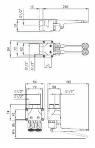
Specialized foot tap with 1/2 "connections for cold and hot water. The faucet body is made of chrome-plated brass. The recommended method of mounting the product is wall mounting. In addition, the foot battery has a built-in vandal-proof system. The range of water temperature that may be approved for use is 5-70 ° C, at a water pressure of min 0.5 bar - max 6 bar.
