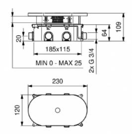
The 2545 electronic faucet is made of brass covered with a chrome layer. A mounting box made of plastic is attached to the set. The internal parts of the mixer are made of anti-scale parts. The offered faucet has a one 3/4" cold or mixed water connection. The 2545 shower tap is available in two power options:
