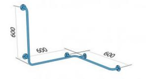
Right handrail for the bathtub left-hand shower mounted to the wall 600x600x600 mm long, made of carbon steel tube with a diameter of 25 mm powder coated white. We use this type of handrail in the bathtub and shower area.
