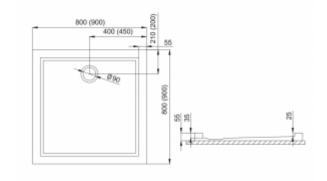
Non-threshold shower trays significantly improve the comfort of using the shower for disabled people in a wheelchair. Installation at the floor level causes trouble-free rolling of the wheels onto the tiles and shower tray threshold. The non-slip surface improves the safety of people using the shower equipped with a no-threshold shower tray.
