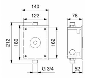
Flush-mounted electronic flush faucet. The tap has a connection G3/4. The outer casing of the product is made of AISI 304 stainless steel, with a chrome finish. It is worth adding here that the correct operation of the tap is possible only when connected to water free of impurities. An indispensable element for the correct operation of the product is a filter (must be installed by yourself).
