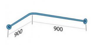
Angular shower curtain rail made of white powder-enamelled carbon steel (anti-corrosion primer was used for enamelling). The 900x900 handrail is intended for wall mounting in the shower area where, in combination with a non-threshold shower tray, it is an optimal solution for the disabled.
