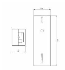
$Soap\ or\ disinfectant\ dispenser\ in\ a\ stainless\ steel\ case,\ elbow.\ Matte\ surface\ finish.\ The\ material\ from$ which the dispenser was made guarantees long-term corrosion protection of the coating. The construction of the dispenser is vandal-proof closed with a key and the edges are rounded. The soap is refilled from the bulk package after opening the housing. It does not require expensive soap cartridges. The soap tank has a capacity of 500 ml.
