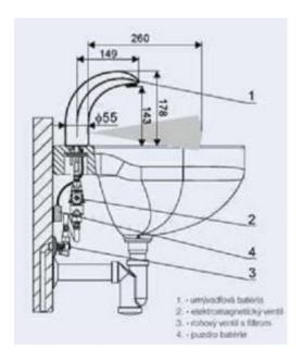
Electronical sink battery, Possibility to conect hot, cold and premixed water. High class materials used for the batteries provide long-lasting, flawless work and also makes the product very vandal-resistant. Designed for public facilities.
