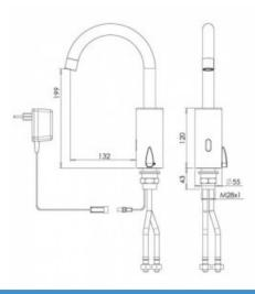
Contactless sink battery with mixer. Equipped in mixer. Designed for public facilities and homes.
