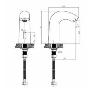
Electronic basin faucet. It can be connected to hot, cold or mixed water. High-quality materials used for the production of time batteries ensure its long-term, trouble-free operation, and also make it extremely vandal-proof. Designed for public utility rooms.
