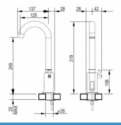
Electronic mixer with a mixer for two 1/2 &HASH39; connections for cold and hot water, adapted for installation on a washbasin. The battery is available in two power variants:
