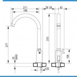
Electronic mixer with a mixer for two 1/2 &HASH39;connections for cold and hot water, adapted for installation on a washbasin. The battery is available in two power variants: • 230V / 6V DC power supply (built-in motor) - Product ID 9193R
